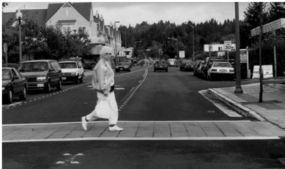
Raised Mid-Block Crossing
