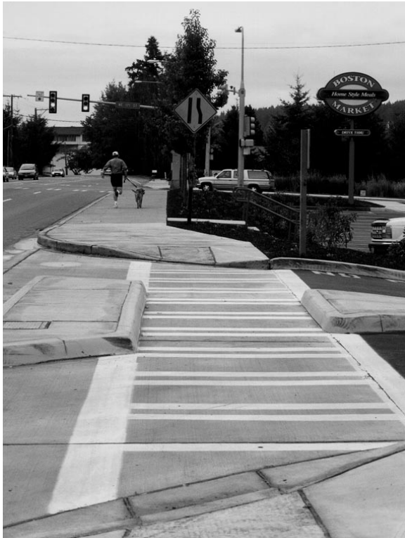
Site access should be well delineated to minimize conflict between pedestrians and vehicles.
