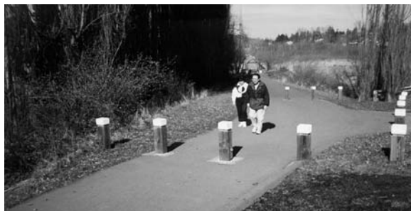
Bollards provide access control at points where pathways join or cross roads.
